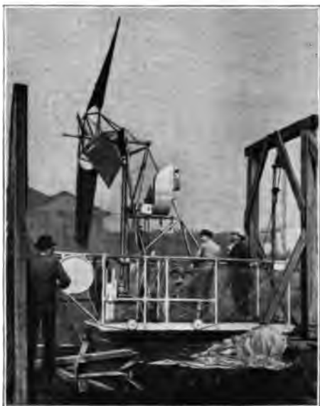
SCREW-PROPELLER AND CAR OF THE GERMAN AIRSHIP "PARSEVAL"
