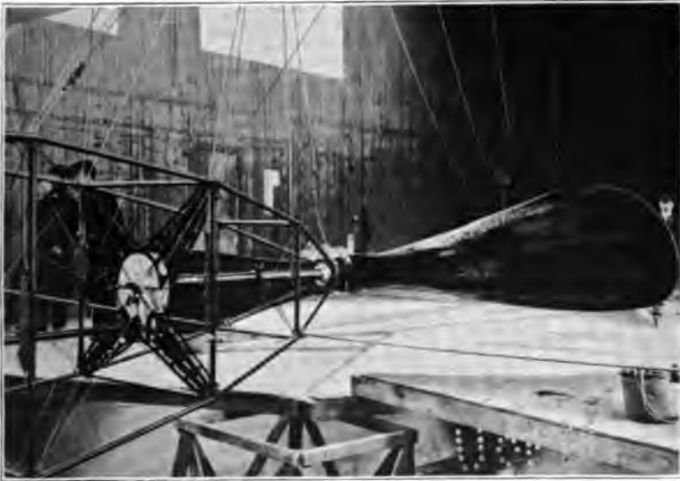
THE SCREW-PROPELLER OF THE "BAYARD-CLÉMENT"
