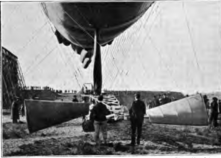
THE SCREW-PROPELLER OF THE "VILLE DE PARIS"
